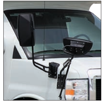
Front 6.75" x 9.75" flat & 6" x 3.5" convex mirrors with left and right cross-view mirrors
